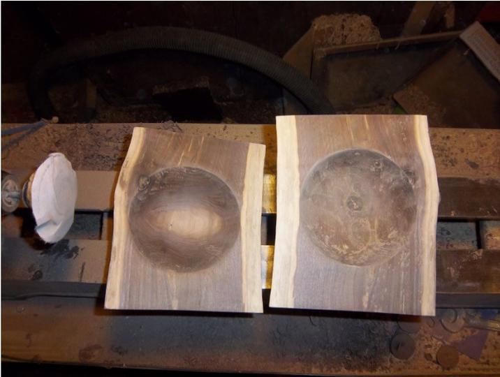
Using sandpaper on a cushioned dish sander attached to the head-stock of the lathe with a chuck, the final sanding can be accomplished. The work goes surprising quickly. The faces and the ends can be cleaned up at this point as well.
