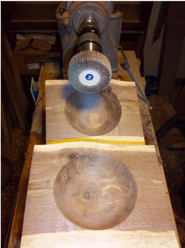
Using a sandpaper wheel [60 grit] on the head of the lathe held by a chuck, the bottom of the bowl can be cleaned up nicely. Again, be careful to maintain the curvature of the cut you put in with the gouge with the bowl was on the lathe. The sandpaper wheel [60 grit] on the head of the lathe is show below. The now cleaned out bowls are also shown.
