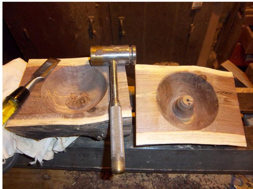
The image below shows both cones removed with the use of a chisel.
