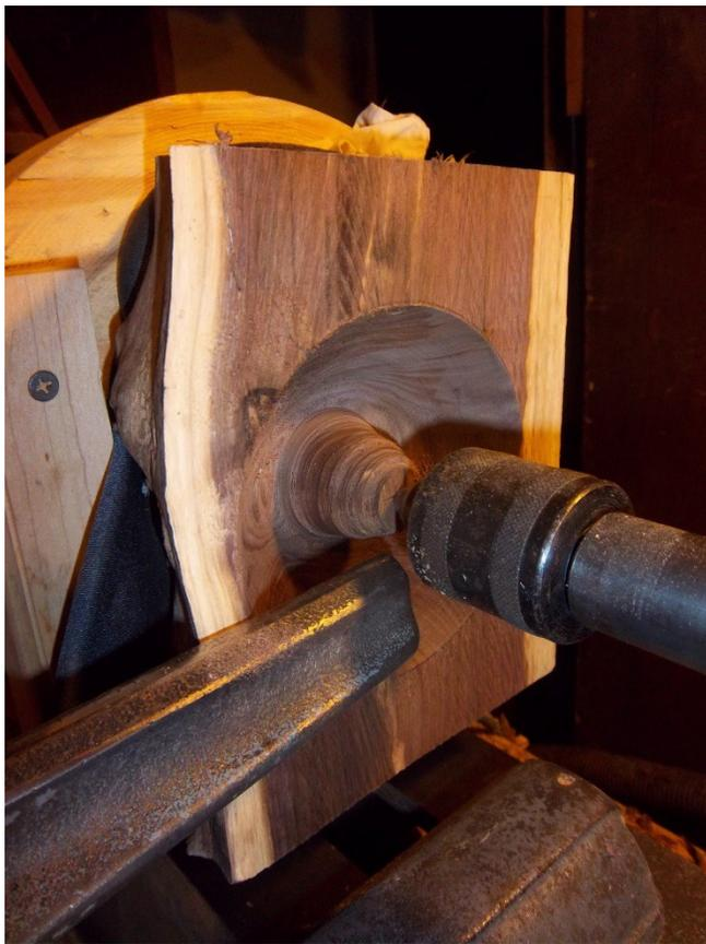
Now the fun begins! Start turning out as much of the bowl as you can but leave a reasonable cone around the tail-stock for support. I have found it is better to leave more of a cone than less. This is so the cone does not split and your piece goes flying off the lathe. And getting rid of that cone is not that difficult as you will see. The image below shows the piece turned about as much as you can.
