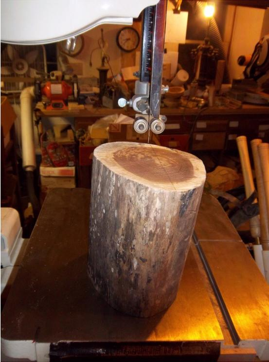
Begin by finding a log or branch of appropriate size. Here is a black walnut log of about 8 inches in diameter and approximately 10 inches long. It is on a band saw to be cut in half along the long axis through the pith.
