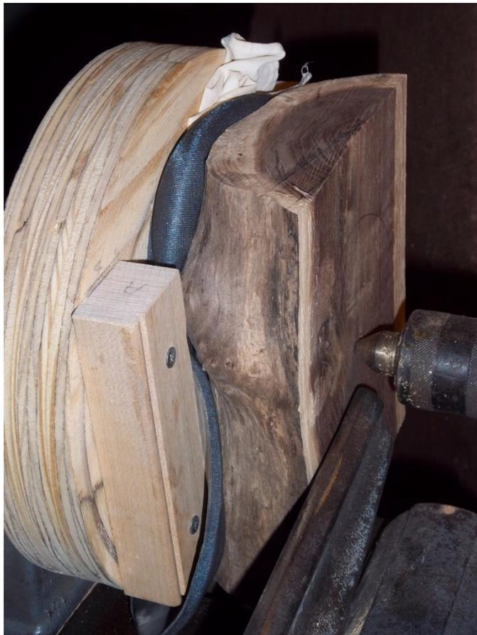
Another view of the log “pinned” into place and ready for turning.
