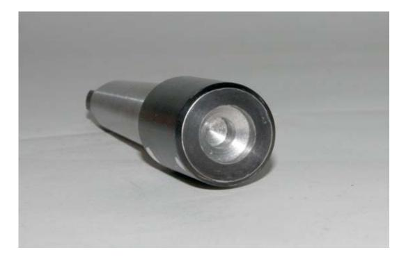
The article stated to glue the router bearing into the hole. I made the hole deep enough for this, but then had second thoughts. If the router bearing seizes, I did not want to have to part off a length of the arbor. I decided I wanted to have the bearing to protrude from the arbor so it can be gripped with a pair of pliers to remove.
