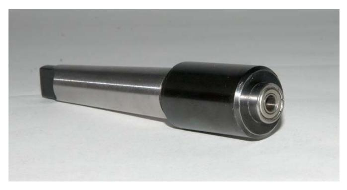
I used a 1/2in OD x 3/16in ID router bearing from an old router bearing kit.
