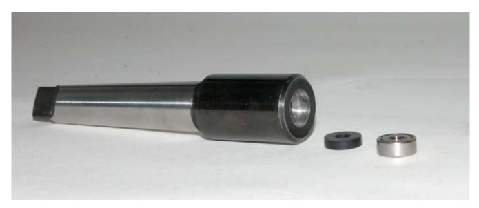
The bearing mounted in the end. I then used some gel (thick) CA glue to hold this in place. No picture of this part since it looks about the same with some CA glue at the end.
