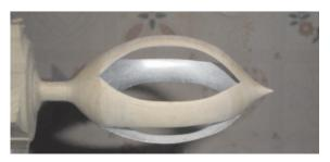
After the inside is complete, each of the four pieces is rotated 180° moving what had been the inside, to the outside. Pairs are glued and clamped. The surfaces to be glued must be flat. If necessary they can be flattened on a piece of sandpaper laying on a flat surface. Glue should be applied to all surfaces, but used sparingly. If the RubNBuff is not dried, glue squeeze-out will discolor it.
