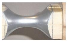
An Inside/Outside turning is made from four square pieces of wood cut to an equal length. It is important that each of these piece are as square as possible. For this example, each piece of wood is 5/8" x 5/8" x 4".
