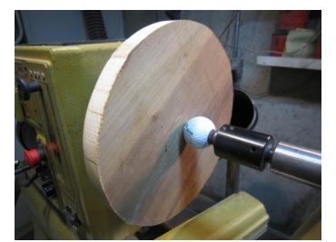
The piece is now mounted on the lathe and the tailstock is brought up for support. Notice the golf ball added to the live chuck. This prevents dimpling the surface
