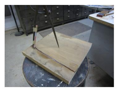
I started with a dry piece of Poplar. There are prettier woods, but this was used because I have a 10" wide plank that has been in my shop for years. I use a compass to mark a 10" circle which I will cut on the bandsaw. (Notice the crack in the wood. I feel that the crack does not go all the way through so I have applied super glue. This plate will be painted later, so the crack adds character).
