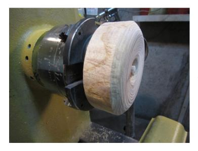
I'm going to use a jamb chuck to hold the plate while turning the other side. I have used a scrap piece of wood to jamb the plate against. The scrap has been trued and sanded.
