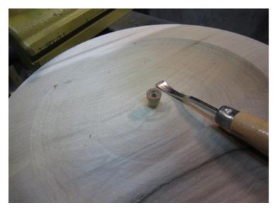
A small carving tool is used to remove the nib. Next step is to sand. I find it useful to mount a sanding pad on the lathe. Turn the lathe on to about 500rpm and hold the plate up against the sanding pad. Easier than trying to hold the sanding pad in a drill while sanding.
