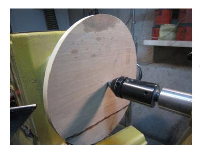
The plate is brought up against the jamb chuck and held in place with the live tail center. Notice the cone attachment. It will fit into the drill hole used for the screw chuck and the piece should be centered on the lathe.
